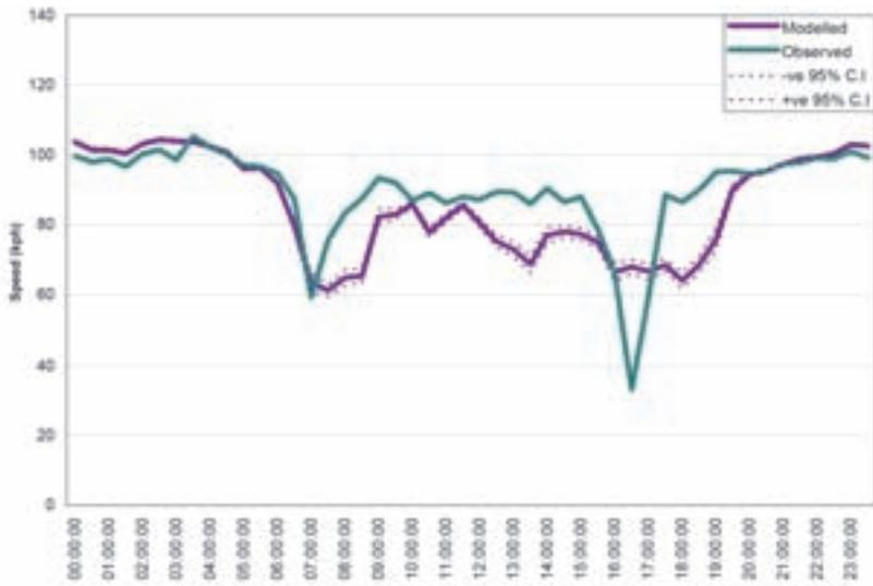
**Figure 3 : Link Speed Validation M4 W of M25 (eastbound)**
